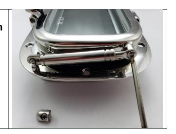
6. Position the clasp of the Stay Arm Piston so that it aligns with the pin on the Portlight and tighten.
