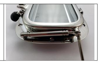
2. Loosen and remove the screw that is holding the piston of the Stay Arm to the Portlight. This will remove the clasp around the pin on the Portlight
