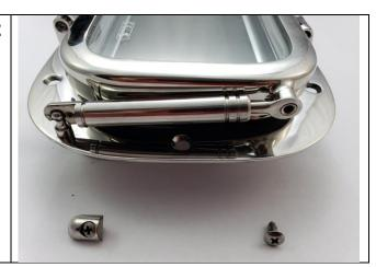
5. Insert screw and tighten the shaft of the Stay Arm to the Portlight
